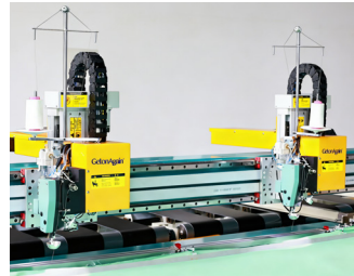
15cm自动升降机头 Lifting sewing head up to 15cm
